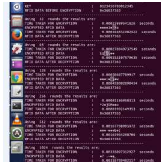
Fig7: Encryption and decryption time of RF based TEA algorithm using python software.
