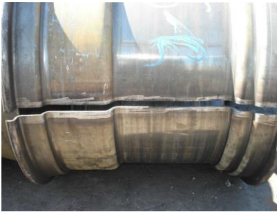
Fig. 7: Breaking of the workpiece basic material.
