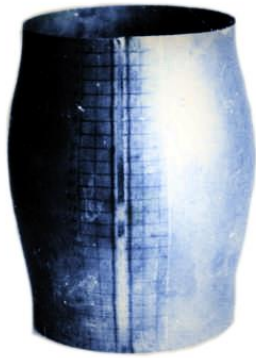
Fig. 14: Cylindrical sample after stamping.
