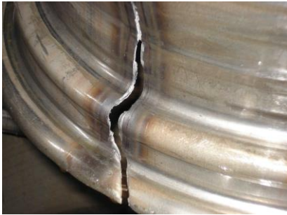
Fig. 4: The weld seam rupture on the wheel rim.
