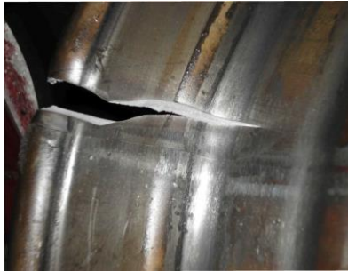
Fig. 6: Combined rupture of the weld seam and the weld zone.
