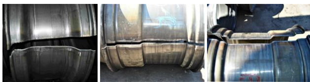
Fig. 15: The samples of wheel rims cylindrical workpieces after test.
