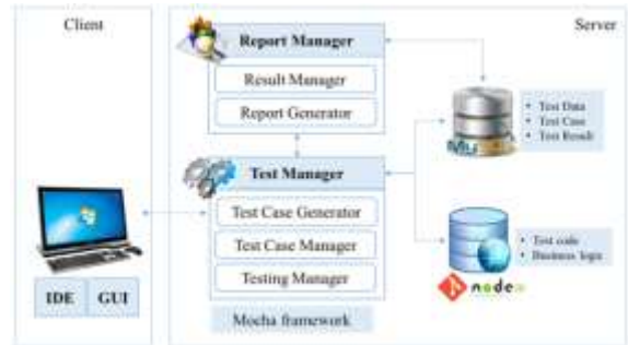
Figure 3: The overall configuration of the system
