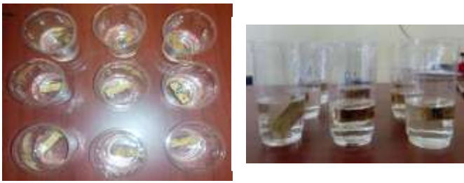
Fig. 4: Water absorption testing
