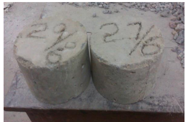
Fig. 9: Specimens of HVSC before Cantabro test.
