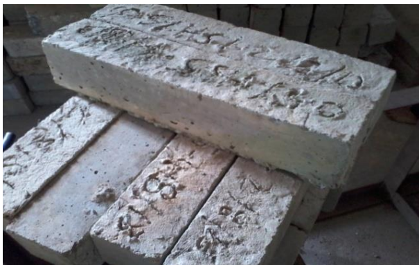
Fig. 5: Specimens of HVSC with and without Fibres.
