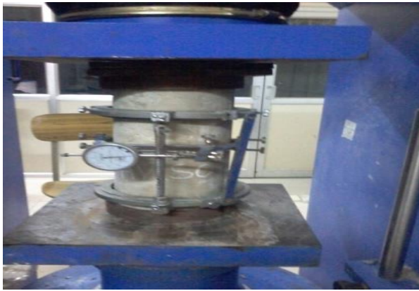
Fig. 3: Test Setup for Finding Young's Modulus Velocity.
