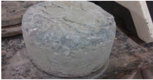
Fig. 10: Specimens Of HVSC after Cantabro Test.
