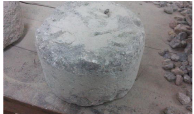
Fig. 8: Specimen of OC after Cantabro Test Test.
