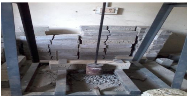
Fig. 6: Impact Strength Test on HVSFSC.
