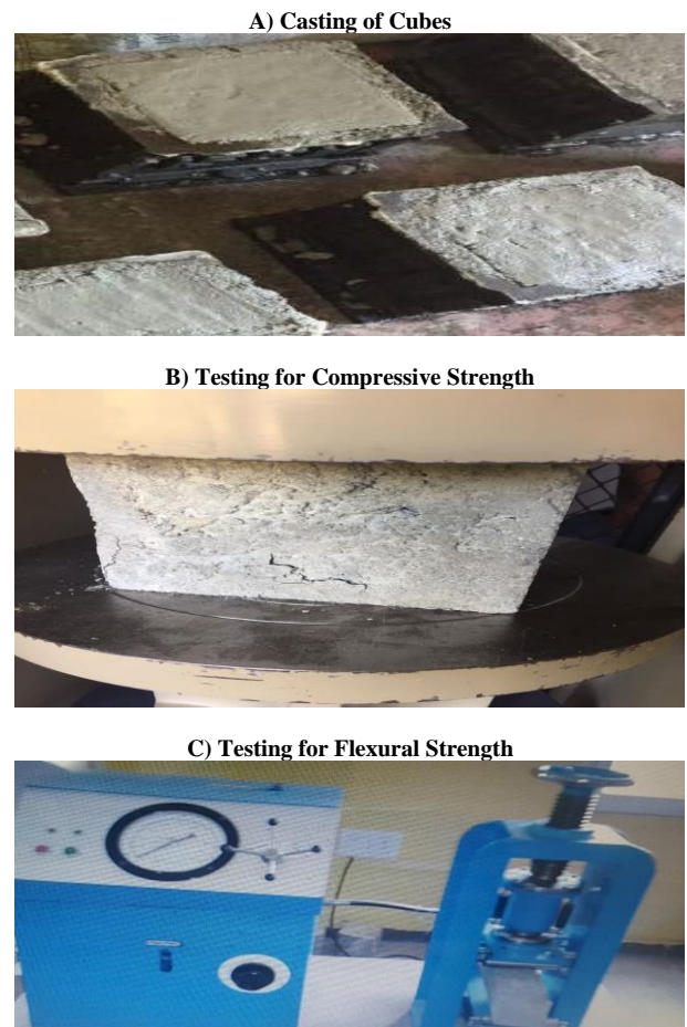
Fig. 2: Casting and Testing of Specimens.
