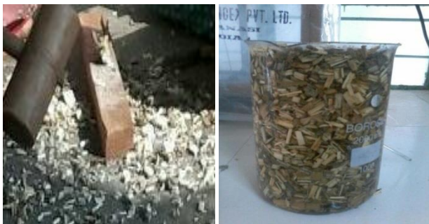
Fig. 1: Cutting and Soaking of Fire Stick Wood.
