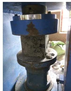
Fig. 2: Casting, Curing and Testing of Specimens Cured by PBC.
