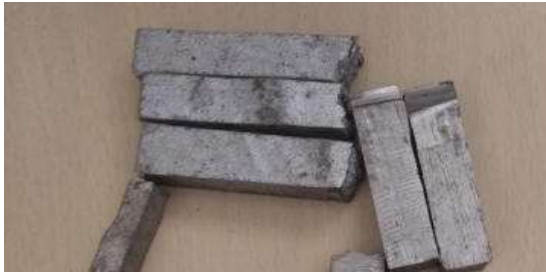
Fig 1: SiC reinforced Al 7005 composite test specimens
