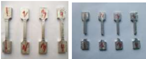
Fig.2: Specimen before Tensile test Fig.3. Specimen after the Tensile test
