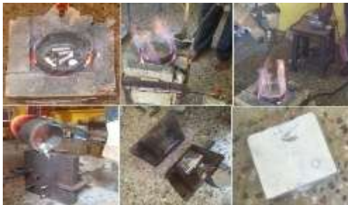
Fig.1: Melting of Al6061 and Stir casting process
