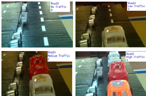
Fig. 7: Shows Four Different Images Captured by a Camera with the Corresponding Output from the Image Processing Algorithm.
