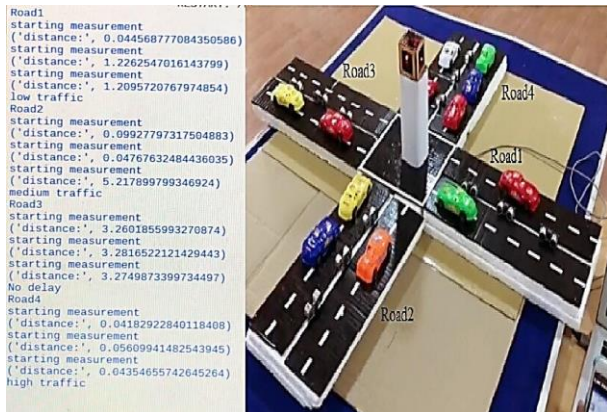
Fig. 6: Output at Python Terminal for the Corresponding Levels of Traffic.
