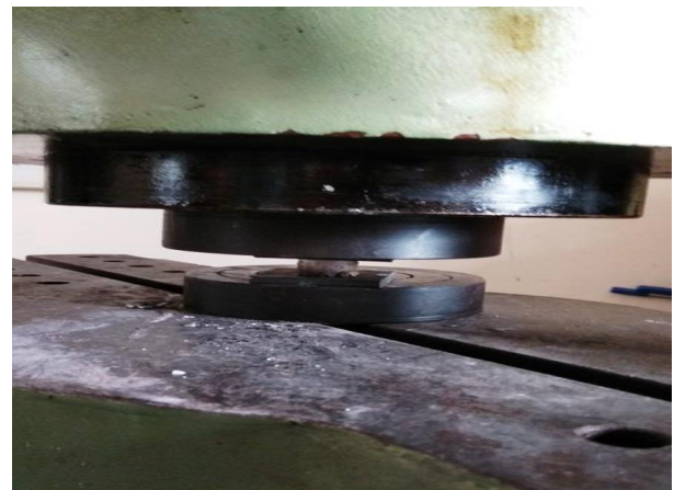
Fig. 2: Specimen Placed In UTM for Compression Testing.
