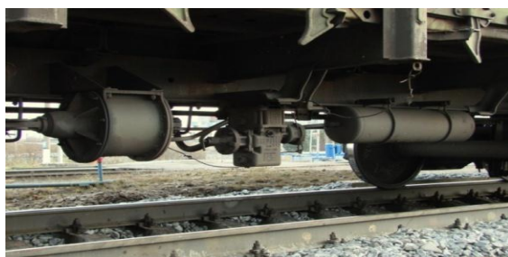
Fig. 1: Air brake system in trains
