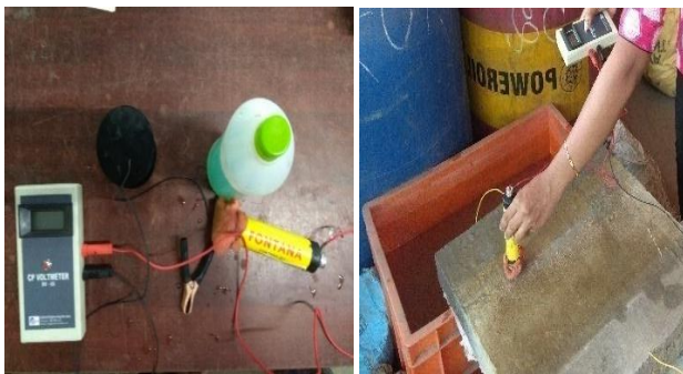
Fig 4: Experimental setup of Half-cell readings
