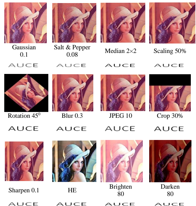
Fig. 3: Attacked Images on the Top and the Corresponding Extracted Watermark Images at the Bottom.
