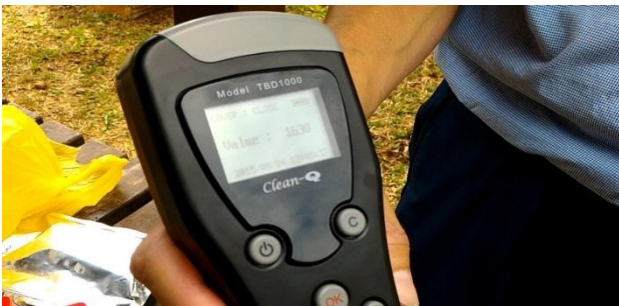
Fig. 5: Portable ATP Detector Shows the ATP Reading for the Water Sample.
