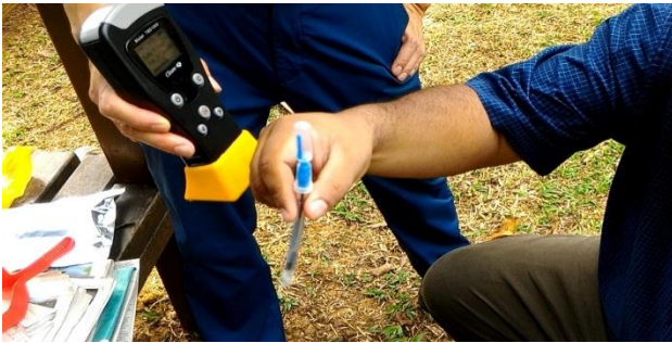
Fig. 4: ATP Stick Is Used to Take Water Sample.
