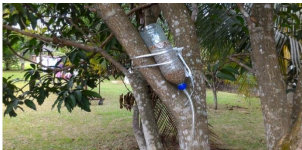
Fig. 1: Top Bottle Serves as the Input for the Water Sample.
