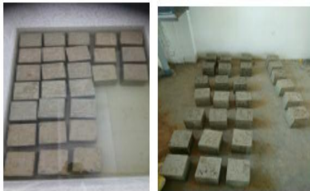
Fig. 3: Specimens are in water cured and at room temperature
