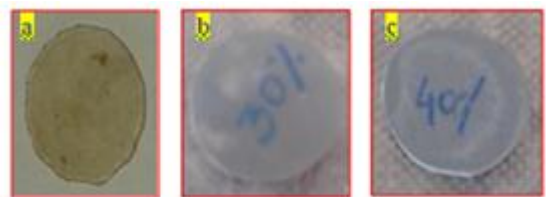
Fig. 3.1: Silicon carbide dispersed polystyrene nano composite sheet
