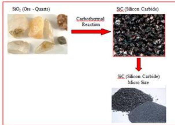
Fig. 2.1: a) transformation SiC nano particulates from Quarts ore
