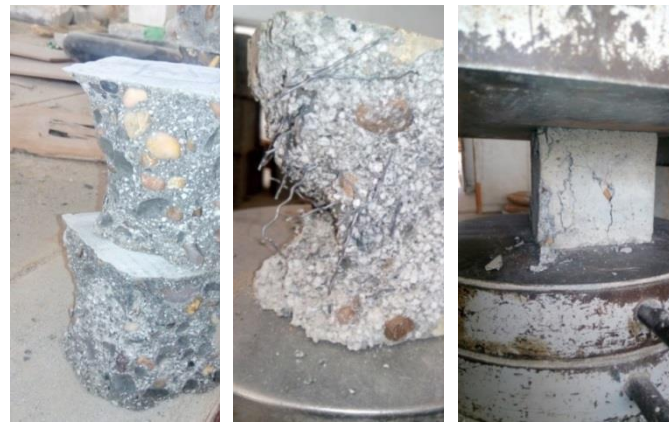
Photo 2: 2a) Compression Failure of Concrete without Fibers for Cube Specimens. 2b) Compression Failure of Concrete with Steel Fibers for Cube Specimens. 2c) Compression Failure of Concrete with Polypropylene Fibers for Cube Specimens.
