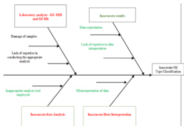
Fig. 7: Cause-Effect Assessment of inaccurate oil type classification from oil spill fingerprints using the Ishikawa Diagram
