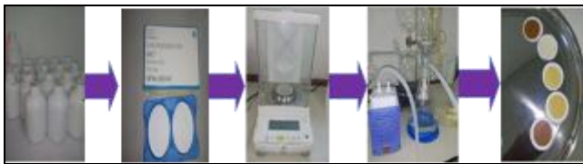
Fig. 4: The Gravimetric Method to analyses the Total Suspended Solid (TSS)
