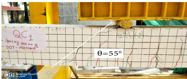
(a) The crack pattern of BWSC-1
