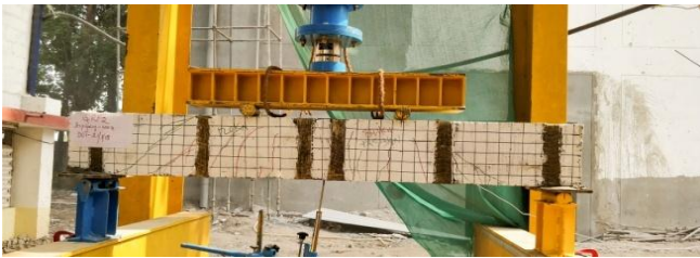
(c) Typically shear failure in BWSRF-3
