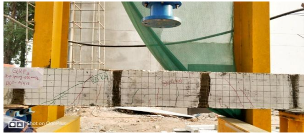
(b) Shear failure in beam BWSRF-2
