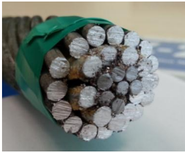
Figure 1: Cross section of the bundle conductor ACSR 330. The inner seven wires are made of ultra-high strength steel and outer 26 wires are made of high conductivity aluminum.
