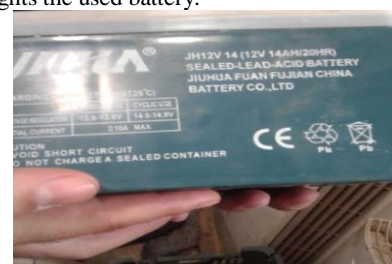
Fig.6: The used battery 12VDC, 14 Amp.hr.
