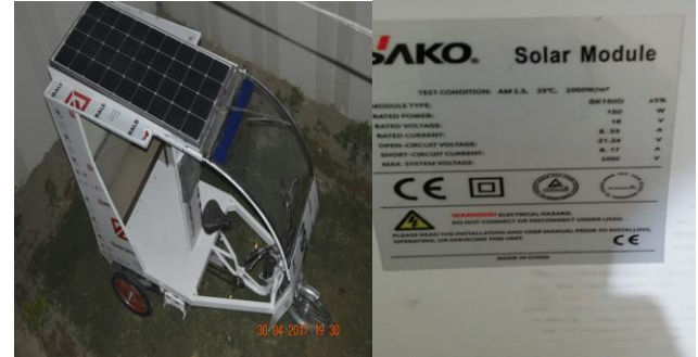
Fig.8: Solar panel is supplying the power to the batteries
