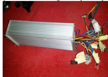
Fig.5: The DC to Three-Phase voltages inverter used.
