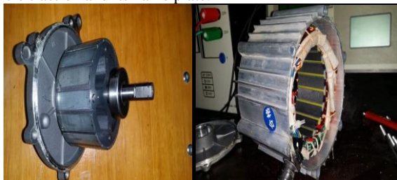
Fig.3: Three-phase synchronous motor for vehicle traction and its name plate.
