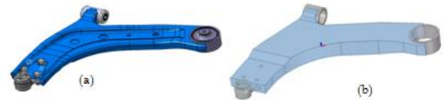
Fig. 2: Current metal stamping (a) and initial concept design (b) of front lower control arm
