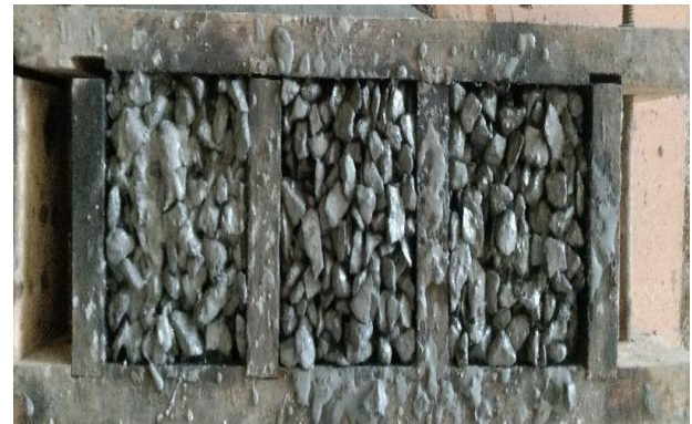
Fig. 1: Casting of cube specimens
