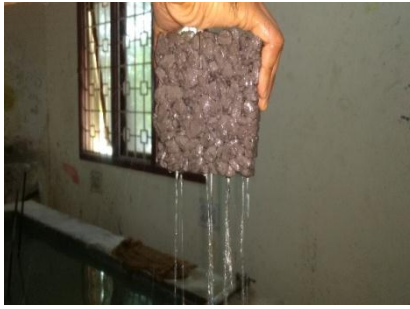
Fig. 2b: Porosity observation in the cube specimen
