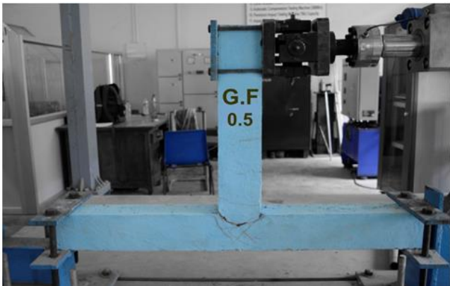
Fig. 7: GFRC specimen crack pattern
