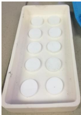
Fig. 2: Sintered bodies of dense MgHA
