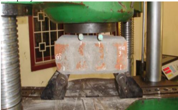
Fig. 2: Experimental set up of masonry prism without mesh embedment
