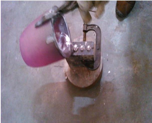
Fig. 2: Pouring of Molten Composite in to the mould
