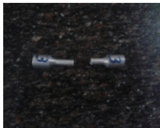
Fig. 6: Tensile.Specimen after testing
