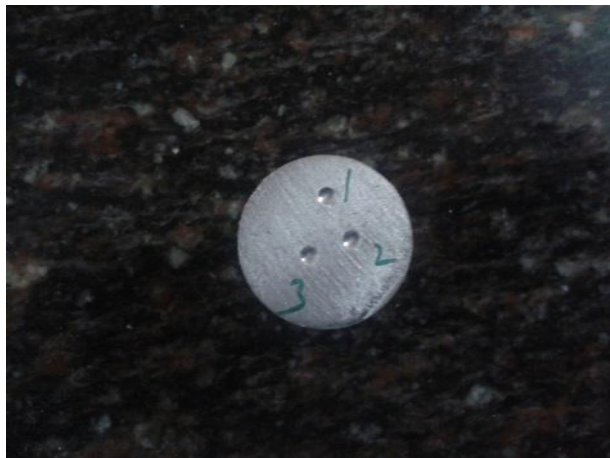
Fig. 9: Hardness. Specimen after testing
