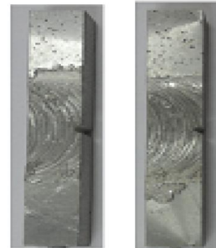
Fig.11 Charpy impact Test Specimen
