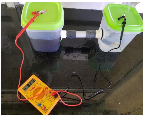
Fig.2: Fabricated Microbial Fuel Cell
