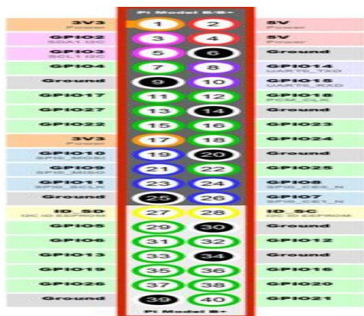
Fig. 3: Pin Diagram of Raspberry Pi.
