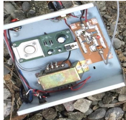
Fig.2: VHF Signal generator and power supply
