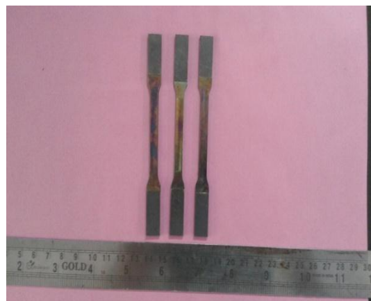
Figure 4: Test specimen—tensile test
