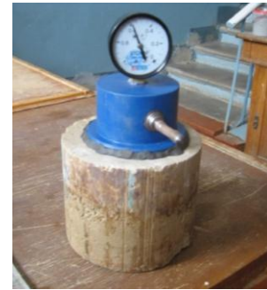
Fig. 5: The device BB-2 for accelerated test of watertightness
