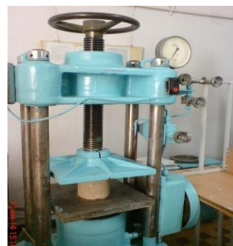
Fig. 1: Tests of soil-cement samples on uniaxial compression on PH-100 hydraulic press
