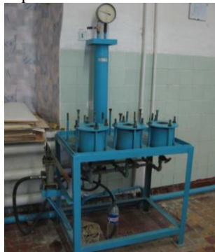
Fig. 4: The device for testing the samples by the method of "wet spot"
