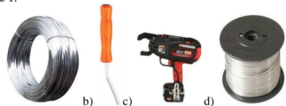
Fig. 1: Armature, crochet tools and materials: a) wire net, b) welded crochet instrument by hand, c) automated reinforcing crochet device, d) wire winding ball
