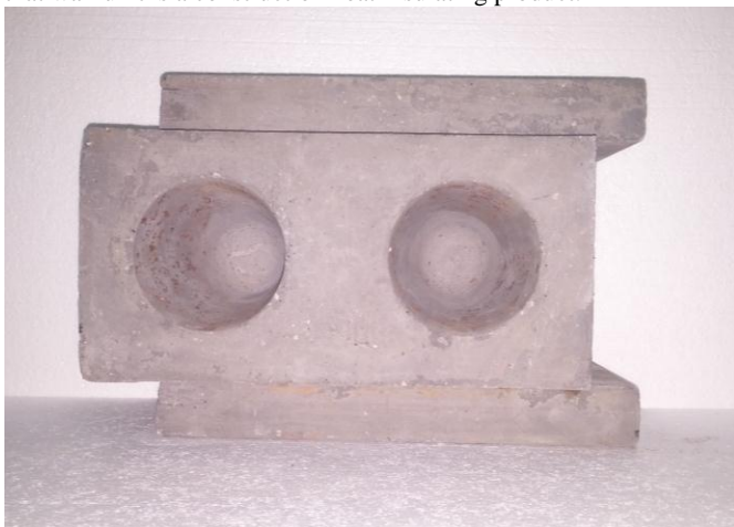
Fig. 11: A wall unit with the ash slag used as a filler.
