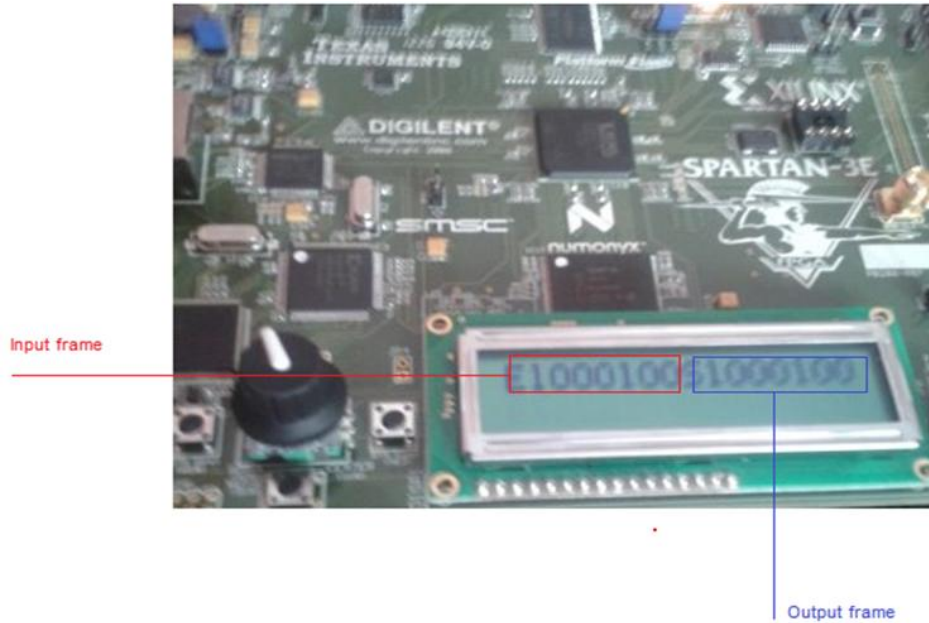
Fig.7: Implementation results on LCD screen of the FPGA Spartan 3E starter
