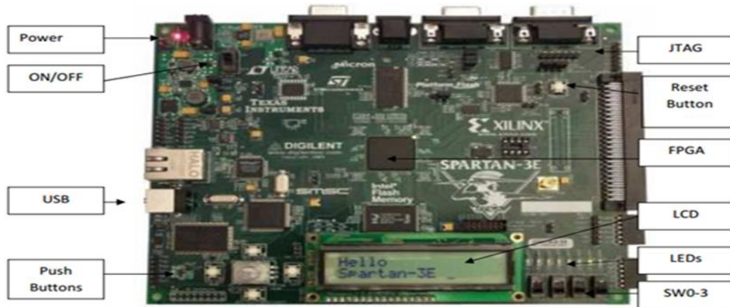
Fig. 4: FPGA Spartan 3E starter board
