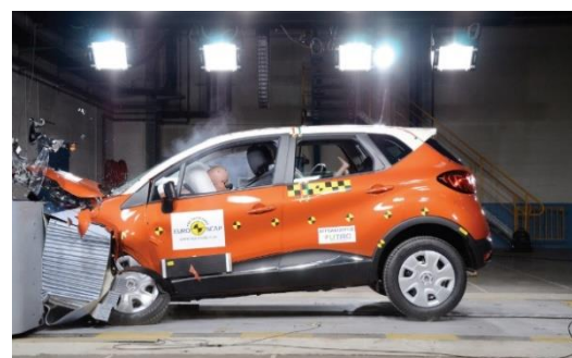
Figure 1. Front Rigid Barrier (FRB) Impact Test
