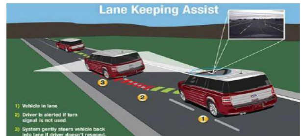
Fig. 6: Lane Maintenance Assist System.
