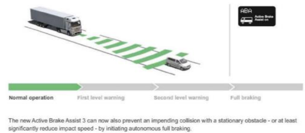
Fig. 7: Operation of Active Brake Assist.
