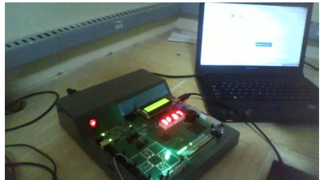
Fig.22: FPGA implementation of transceiver
