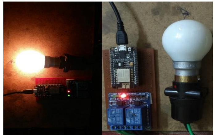
Fig. 27: Interfacing Lamp Through the Relay to Node MCU.
