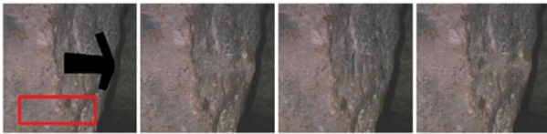
Fig. 7: Results of the Structure-Based Inpainting Approach with Different Values for the Structure/Intensity Weighting Factor. Left to Right: the Input Image, the Output Images Obtained Using K = 0.15, 0.5 and 0.85 .
