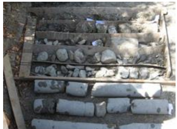
Fig. 4: Drill Core Boxes of PK240+847.
