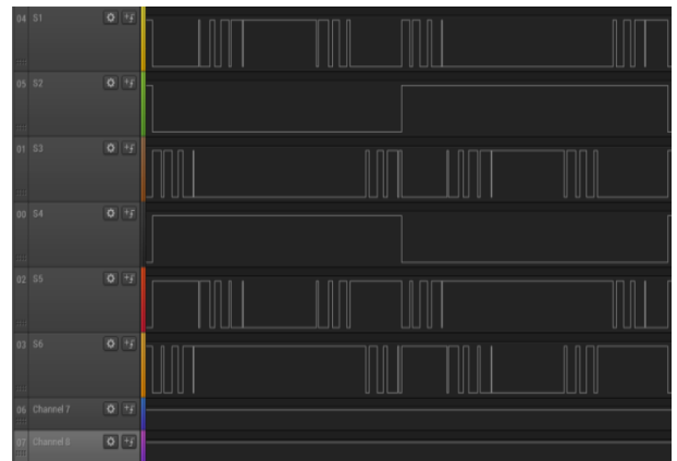
Fig. 11: Signals Synchronizing Test by Saleae Logic Analyzer Via Software (Saleae 1.1.3 Beta).
