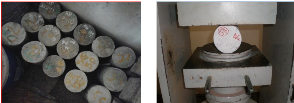
Fig. 4: Casting and Testing of Cylinder Specimens
