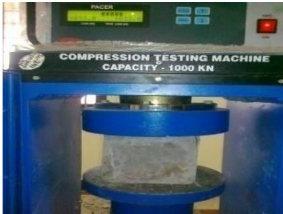
Fig. 2: Cube testing in CTM
