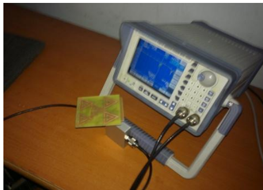
Figure 11(b): Experimental Testing of reduced size RMPA loaded with “STRR” metamaterial structure on Spectrum Analyzer.
