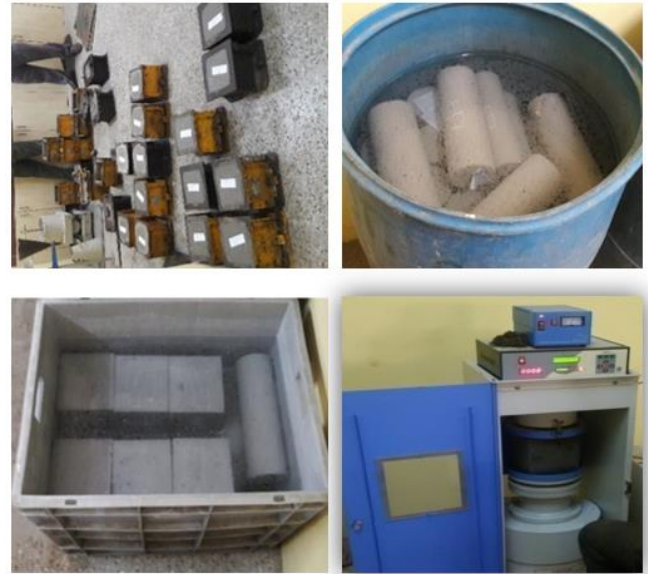
Fig.1: Casting and testing of specimens
